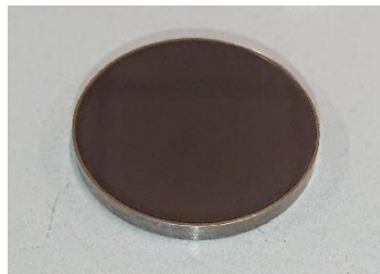
Fig. 1: AlTiN coating onto Ti6Al4V disk realized by SLM.
