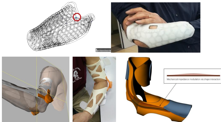
Fig. 1: Top left , Finite Element Analysis of an optimised anatomically-coherent metastructure for multimaterial upper-limb prosthetic sockets, showing region of possible plasticisation – open cells will receive functional materials; Top right , combined prosthesis metastructure and acrylic resin with thermal conductance improved by phase-change material additions; Bottom left/centre , virtual and 3D-printed prototype of a perfect-fit upper-limb orthosis with optimal alignment of hinges functionalised with pseudoelastic alloys; Bottom right : concept of shape modulation for integration of NiTi wires into a compliant orthosis.
