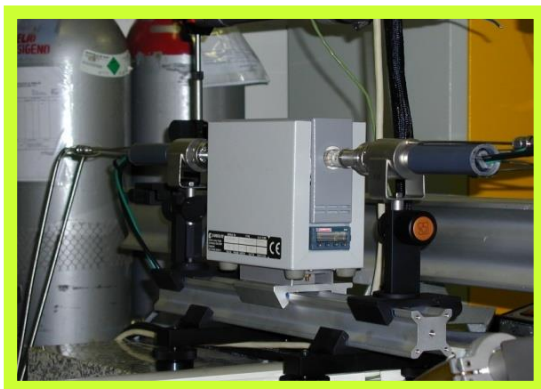
Zirconia sensors to control and measure the Oxygen Partial Pressure
