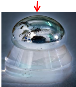
Liquid metal sample on sapphire crucible (Large Drop method)
