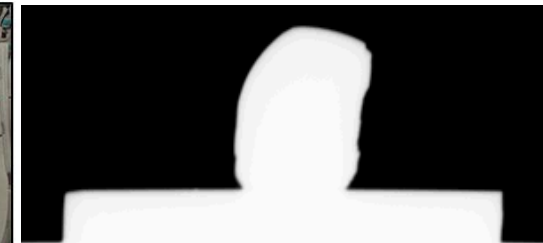
sessile drop during test ( \theta < 90^{\circ} )
