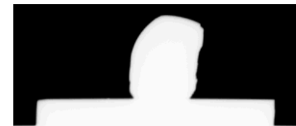
Example of sessile drop during test ( \theta < 90^\circ )
